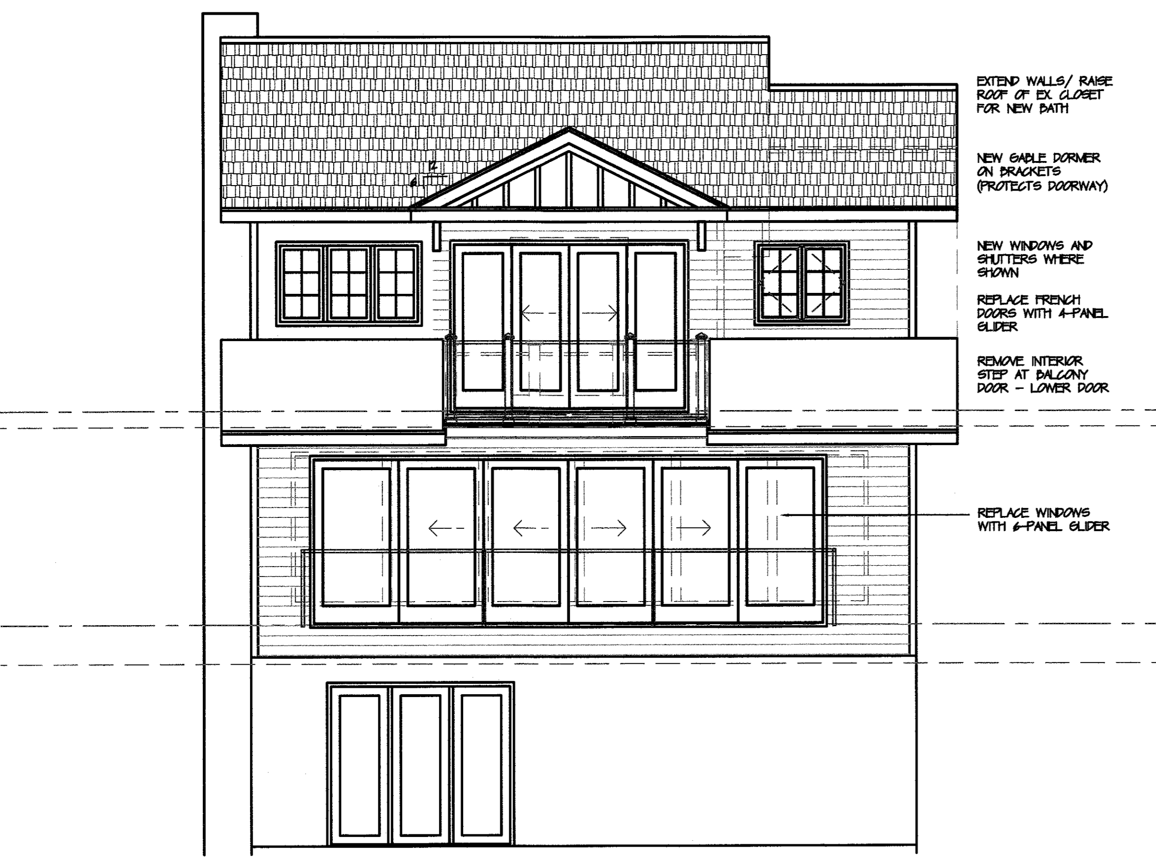
3 REAR ELEVATION SCALE: 1/4" = 1'-0"
