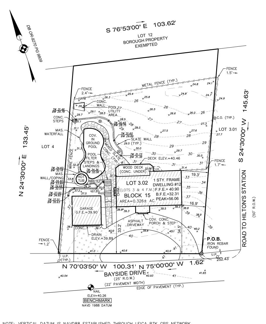
NOTE: VERTICAL DATUM IS NAVD88 ESTABLISHED THROUGH LEICA RTK GPS NETWORK PREPARED FOR: TWO RIVER ENGINEERING
